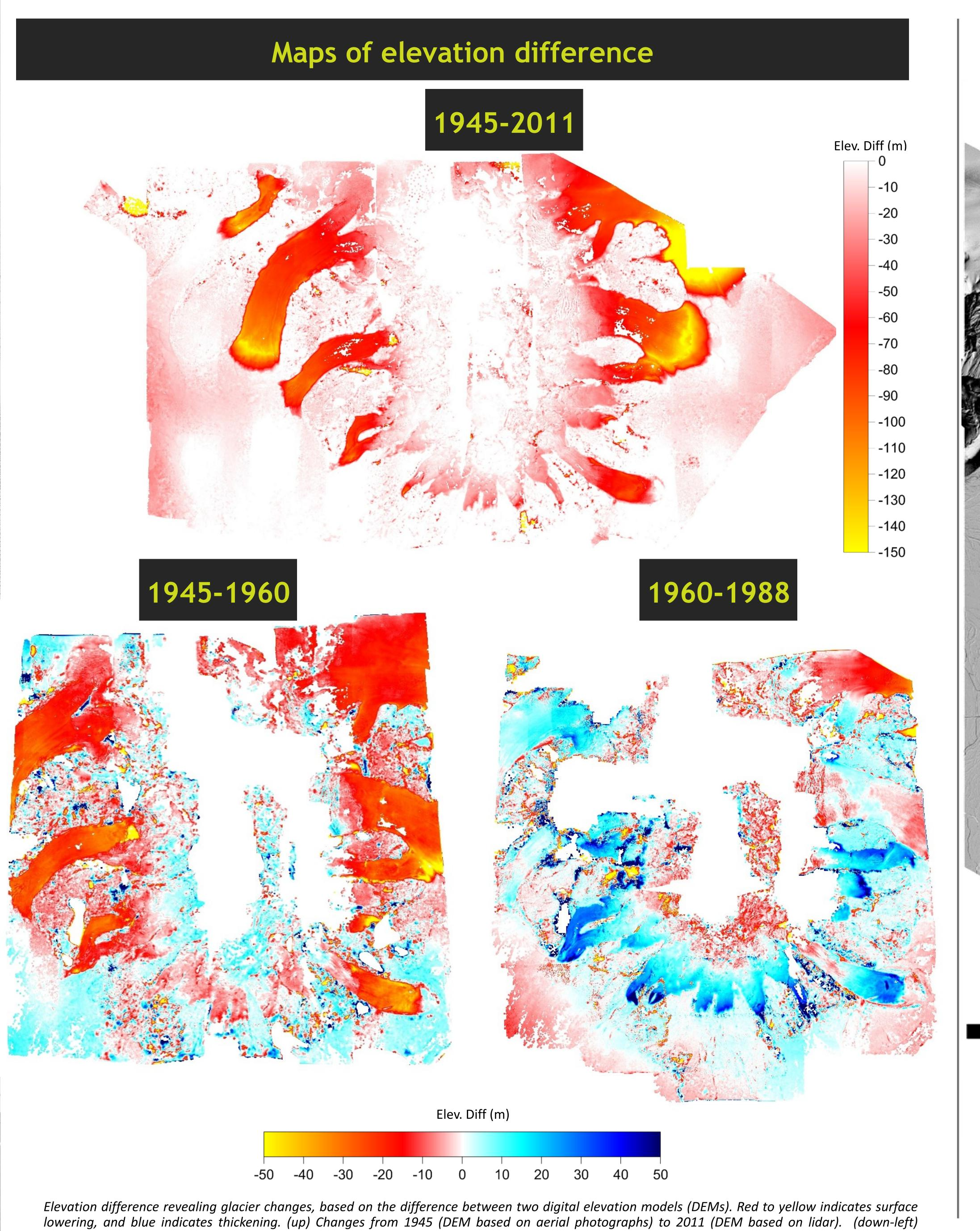
Changes from 1945 to 1960 (DEMs based on aerial photographs). (down-right) Changes from 1960 to 1988 (DEMs based on aerial photographs).
