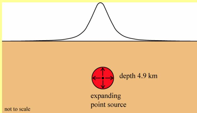
Horizontal movements radiate away from the Katla caldera, interpreted as result of inflation of a magma chamber at 5 km depth beneath the caldera (star).
