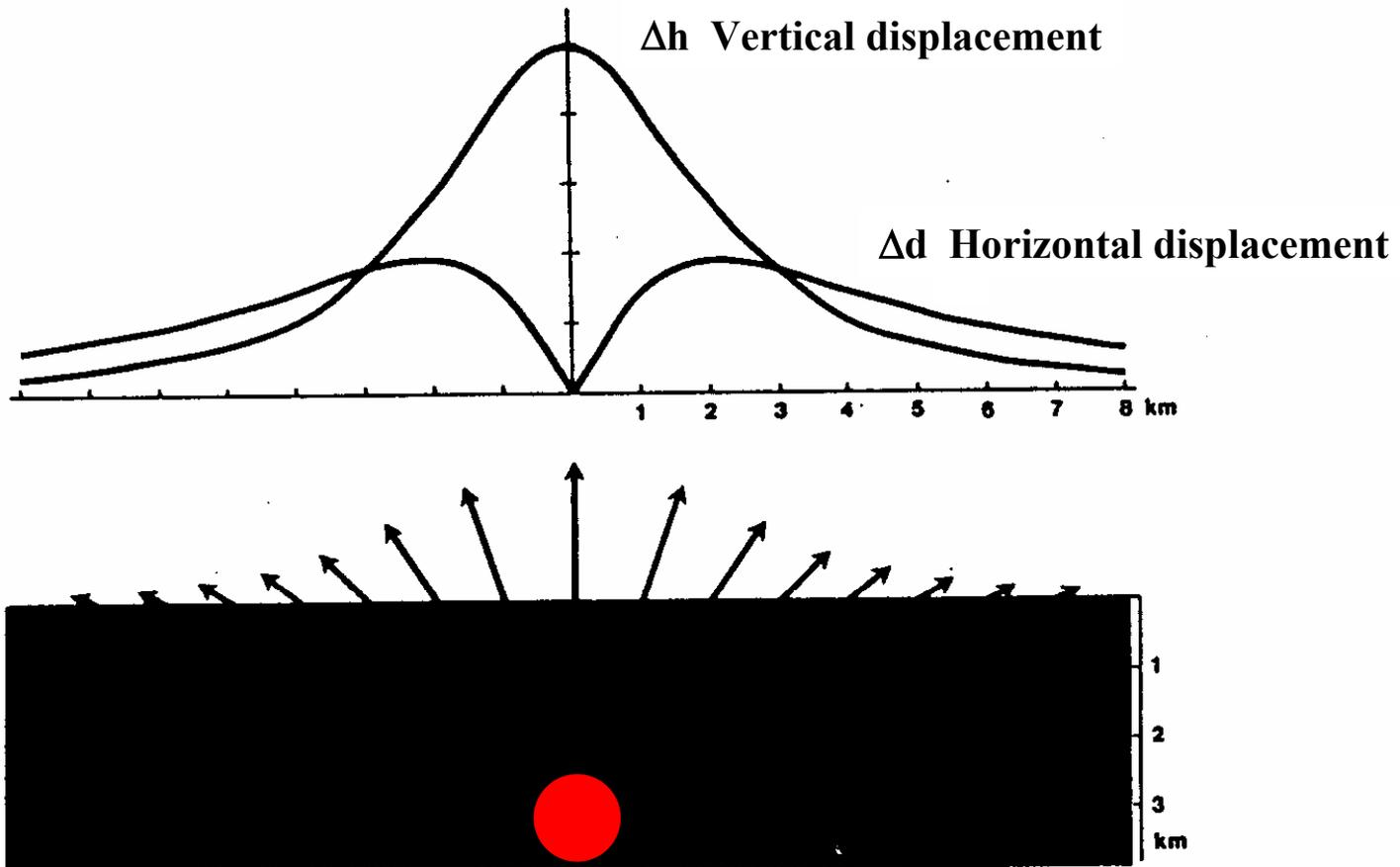
An expanding spherical volume at depth in the crust produces a characteristic pattern of uplift and outward movements at the surface above it (the Mogi-model)
